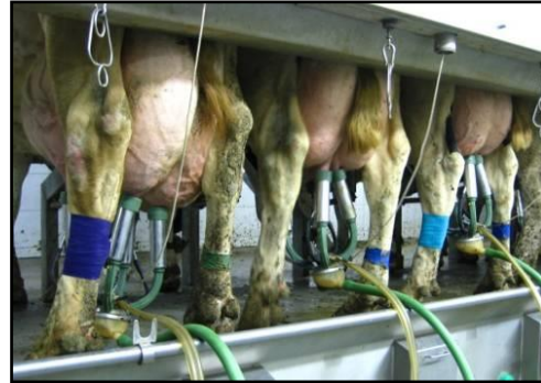
Modern milking parlour: (Left) This parlour can milk 20 cows at a time. (Right) Milking in action: cows have the milking machine attached to their teats.
