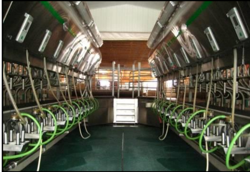
Modern milking parlour: (Left) This parlour can milk 20 cows at a time. (Right) Milking in action: cows have the milking machine attached to their teats.
